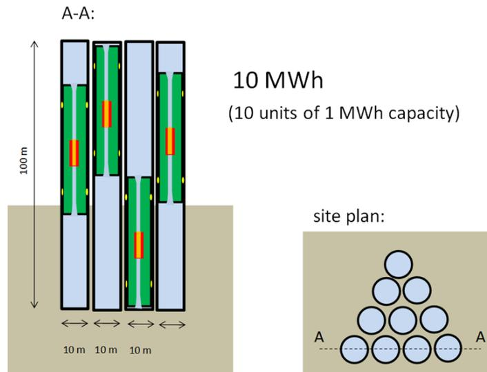
Fig. 2: Cluster of Powertowers with a storage capacity of 10MWh
