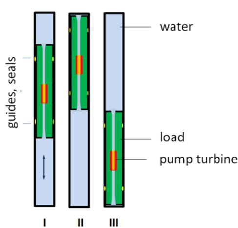
Fig. 1: Principle sketch of a Powertower (I: charging state, II: charged, III: discharged)
