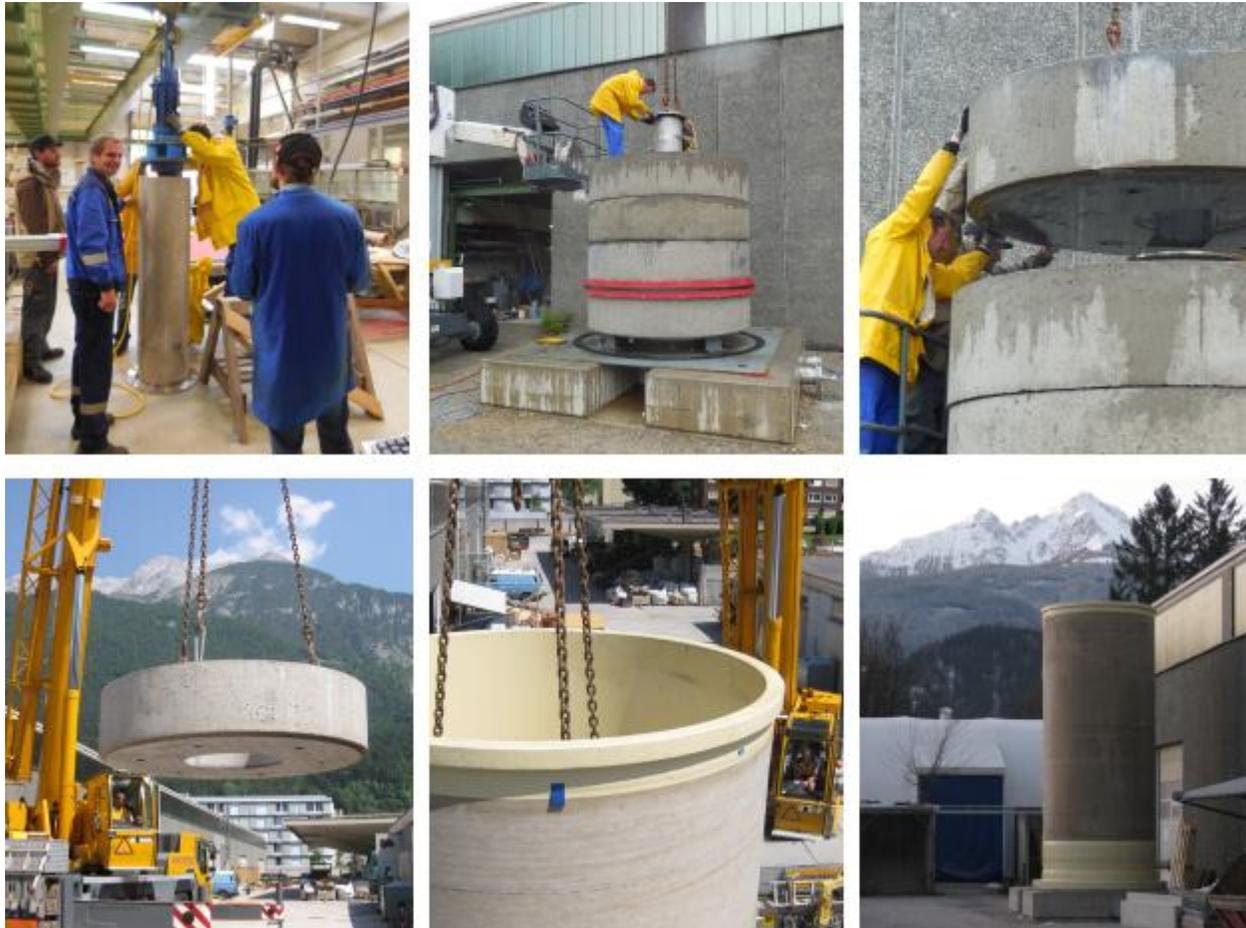
Fig. 4: Construction of model test PT2 with an internal pump turbine
