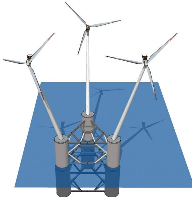
Fig. 6: Floating Wind turbine combined with Buoyant Energy
