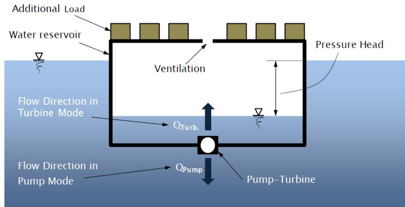
Fig. 5: Principle of Buoyant Energy
